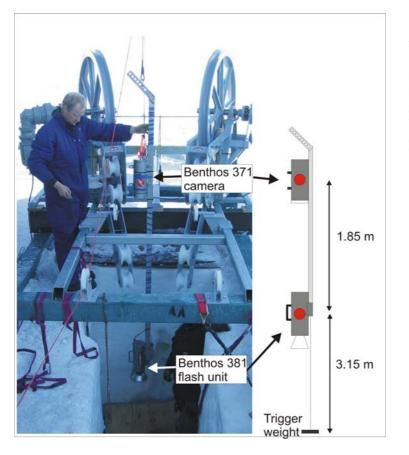
*Figure 3.* Benthos bottom camera system. Note the hole through the ice shelf is covered with plywood in this photo and the trigger weight has not been attached.
