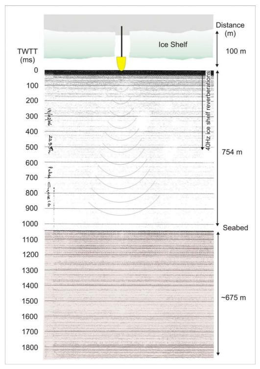
*Figure* 2. 3.5 kHz sub-bottom profile from the analogue chart recorder using a pulse length of 16 cycles. The transducer lies  $\sim$ 2.5 m below the base of the ice shelf. TWTT = two-way travel time (in milliseconds). Note 40 Hz reverberations from the ice shelf contributing to the source function which help to create sub-seafloor acoustic artefacts.
